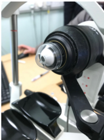
Figure 4: Tomocap mounted on microscope.
