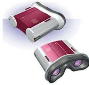
Figure 1: A concept drawing of the proposed handheld binocular OCT device.
