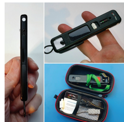
Figure 1: The Arclight: (clockwise from left); side view; rear view illustrating the ophthalmoscope-end, the loupe-end and the solar panel; the complete kit includes a carrying case, charging cable, instructions, two disposable speculae (4.5mm and 2mm) and a lanyard.
