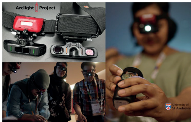
Figure 4: The Arlight binocular indirect ophthalmoscope and simulation eyes for DR and ROP training workshops.
