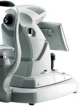
The NIDEK GS-1 Gonioscope rapidly captures quality colour images of the whole anterior chamber angle and the structures therein. A simple alignment process allows for quick and easy auto capture of the whole 360 degree angle.
