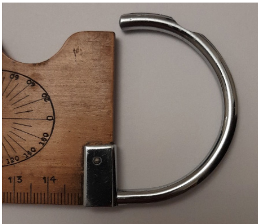
Figure 2: Metal curved component attached to the Preston Frame Rule.
