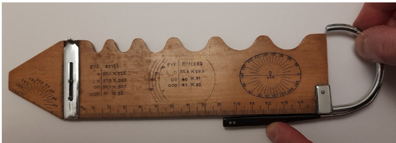
Figure 4: Example of measuring the length of a curved-end spectacle side.
