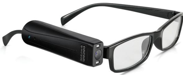
starts very quickly and the user does not need to continue to 'look' at the text as the reading proceeds. For example, while looking at a printed letter I tapped the touch bar. The device started to read, and I was free to get on with other tasks as the reading continued.
