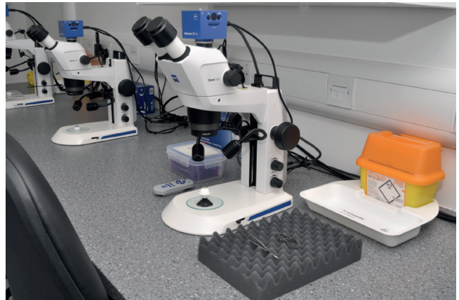
Figure 4: STEMI microscopes connected to a camera for videos.
